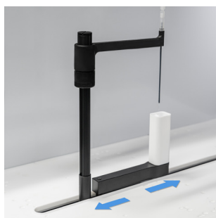
Figure 4. RidingRinse integrated to 4DXW autosampler.
